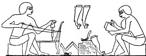
FIG. 34.—Egyptian bow drill.
